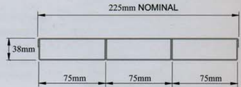
UNDERFLOOR TRUNKING (STANDARD 38mm TRUNKING HEIGHT)
